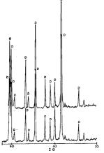
Figure 2:X-ray diffraction diagram of the dolomitic limestone. D:dolomite
